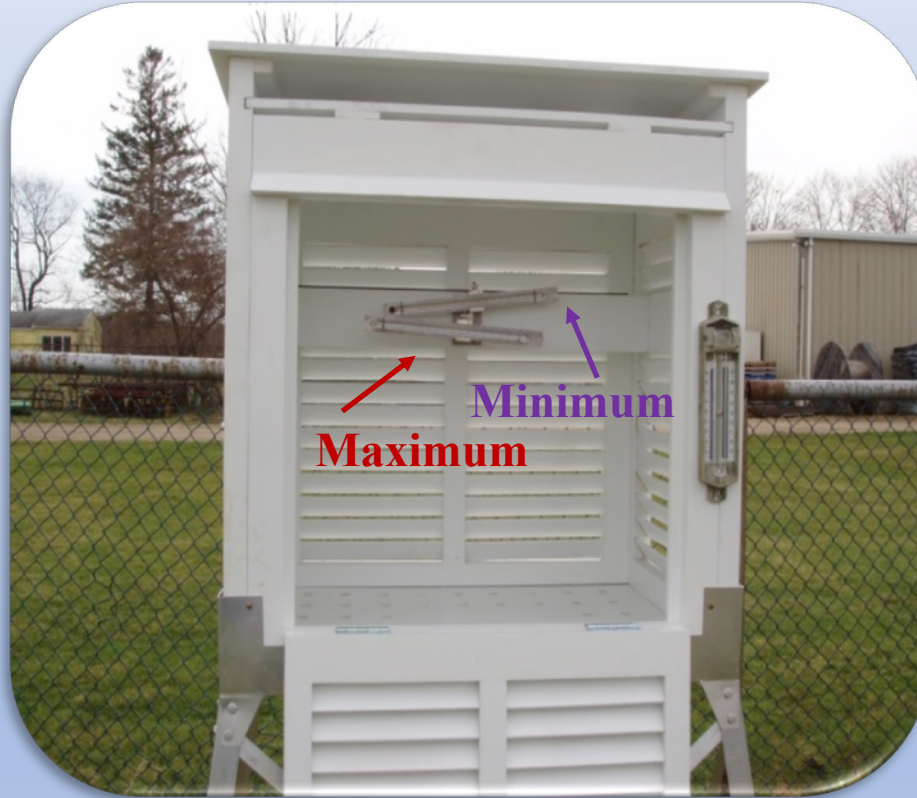
Naturally Ventilated Thermometers Maximum Temperature Mercury Minimum Temperature Alcohol
